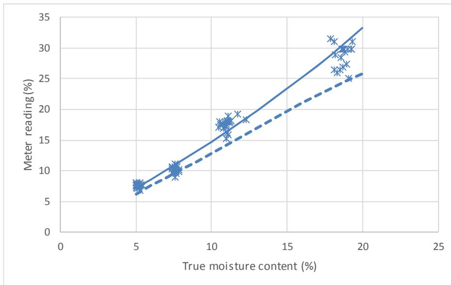
Figure 1. Meter readings using the Carrel & Carrel C201 resistance type moisture meter plotted against true moisture content for 80 NelsonPine LVL samples. Also shown are the quadratic regression model (solid line) and the 5<sup>th</sup> percentile (dashed line).
