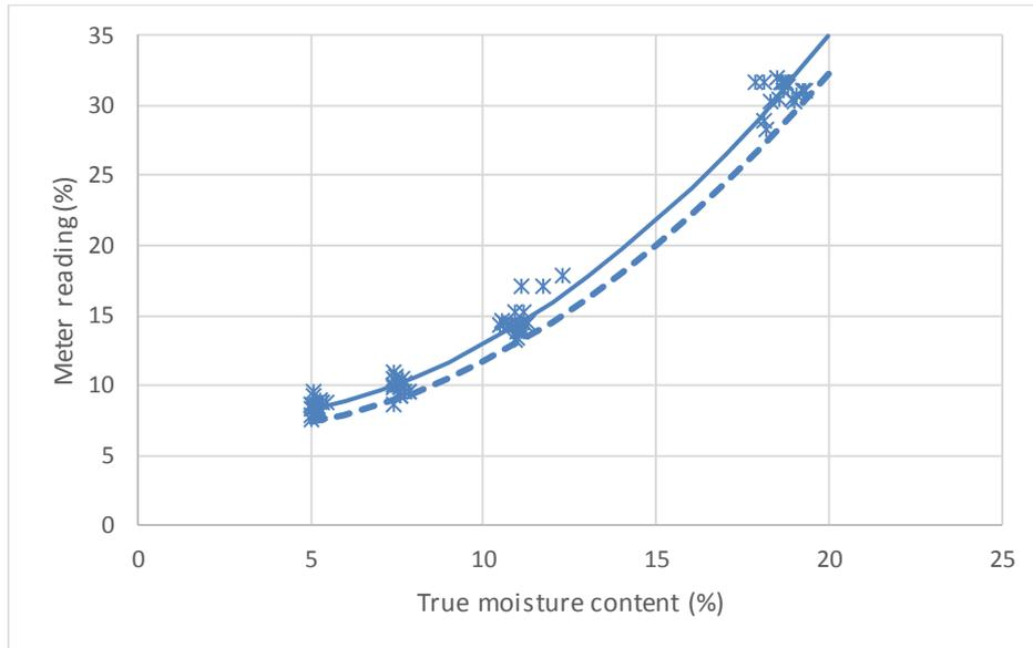
Figure 2. Meter readings from the Wagner capacitance type moisture meter plotted against true moisture content for 80 NelsonPine LVL samples. Also shown are the quadratic regression model (solid line) and the 5<sup>th</sup> percentile (dashed line).
