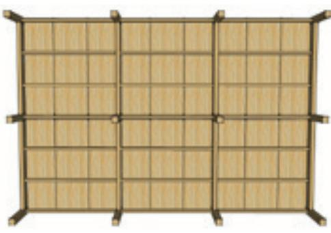
A one-way spanning beam system is materially efficient when the span of the floor system in one direction is maximised. A one-way beam configuration also has advantages for the reticulation of services as they can run parallel to the beam lines.
