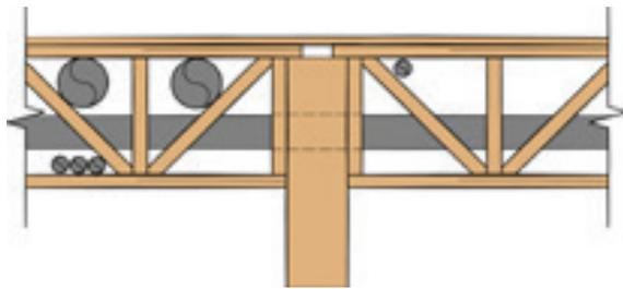
**Varying Grid Spacing** the columns can be spaced closer together in certain areas to allow for a shallower beam depth for services to run beneath. This works well along corridors.
