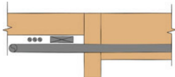
**Suspended Services or Beam Penetrations.** Services can be left exposed suspended beneath the floors and beams or with specific design they can run through penetrations in the main beams.
