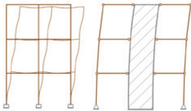
*Idealised displaced shape of Fixed Beam Connections vs. Pinned Connections under Lateral Displacement.*
