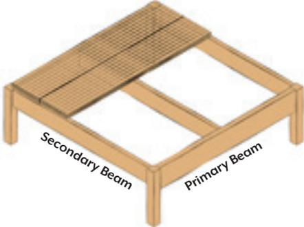
The figure shown is for a two-way beam system where the floor spans between secondary beams. Where there is no secondary beam, the floor spans between primary beams.
