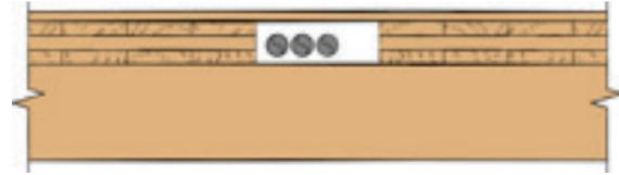
**Thick Topping or Raised Floor** can be used to hide services above the floor panels while leaving the underside exposed.
